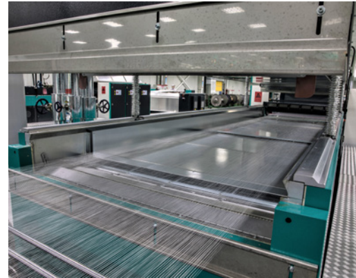
Easily accessible hot air chamber for speedy handling
