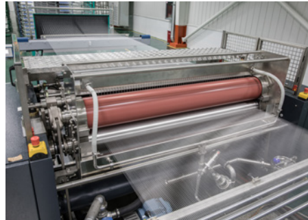
Size box based on one dip double nip and size sprinkling
