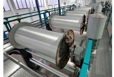
New ergonomic design of beam creel for full-end sizing execution
