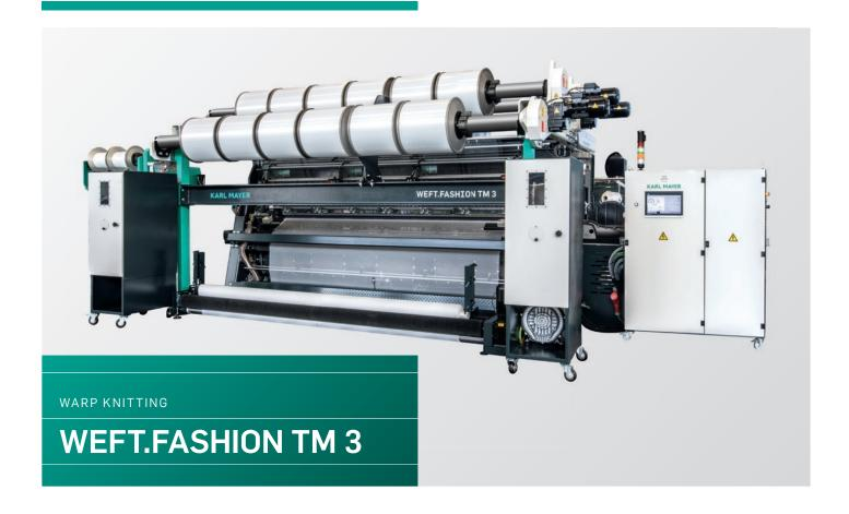
Warp-knitting machine with course-oriented weft-insertion for production of medium-weight home textiles
