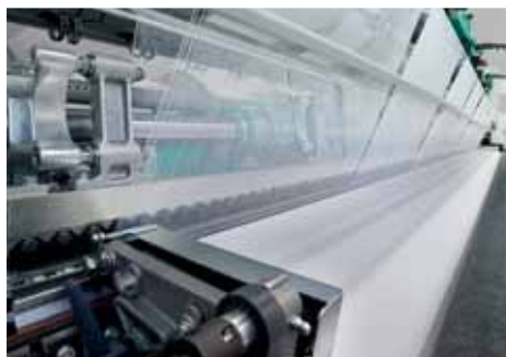
Fabric take-up, electronically controlled 织物牵拉，电子控制
