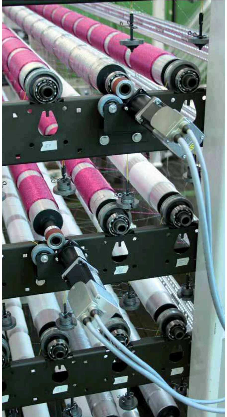
Fig.: Servo system with mounting of the new, active pattern yarn delivery system
