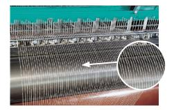
Consistent optimal yarn arrangement: during stopping or starting, the threads between the shaft and the reversing roller may get crossed. During sizing this quite often results in yarn breaks. The automatic detangling function ensures that the thread arrangement is re-established immediately after start-up.
