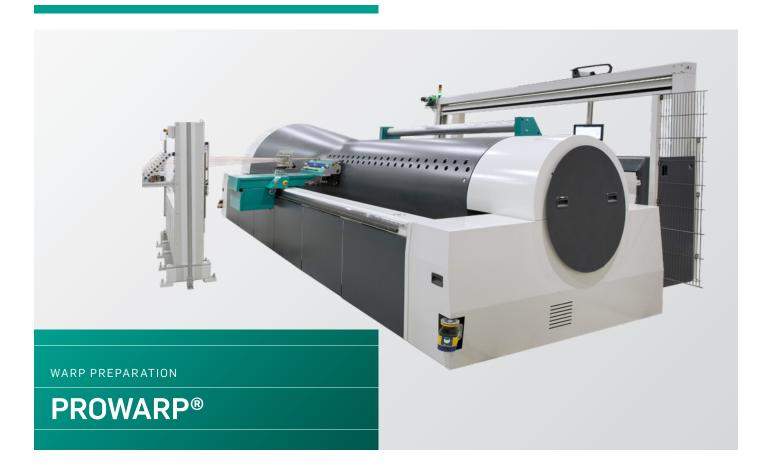
Sectional warping machine suitable for processing all kinds of materials and material combinations equipped with the latest connectivity, measuring and control technology
