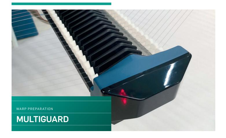
MULTIGUARD for fast and reliable tension measuring and detection of broken ends
